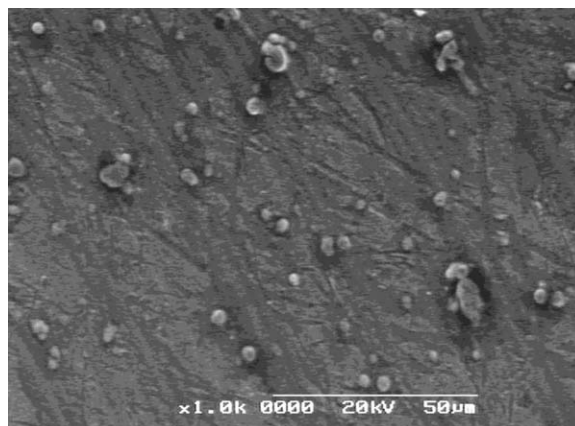
Fig. 7. Scanning electron micrograph of metal-free phthalocyanine particles of specimen F.
